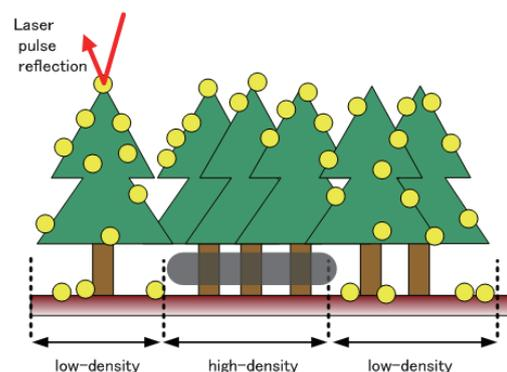
Figure 1. Forest light condition and laser pulse reflection
