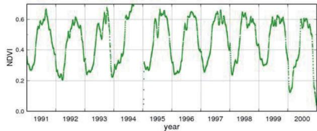
Figure 3. An example of NDVI time series from 1991 to 2000. This time series is composed of daily mean NDVI (8-km resolution) over the land areas of Japan derived from NOAA/AVHRR observation. Daily NDVI values were derived by the temporal window operation (Suzuki and Kondoh, 2005).
