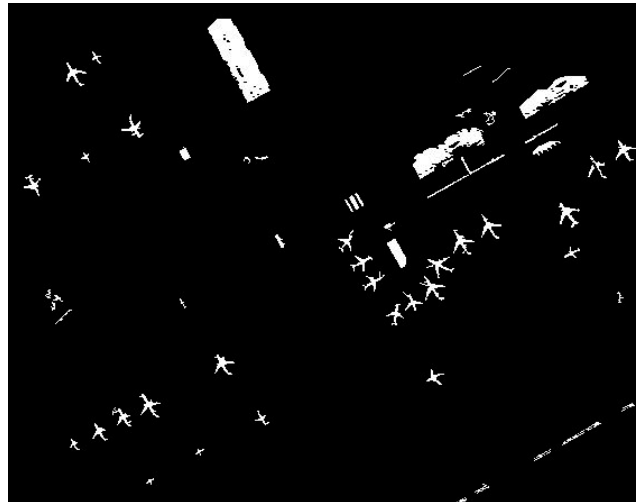
Figure 5. Binarized image after elimination of shadows and small objects
