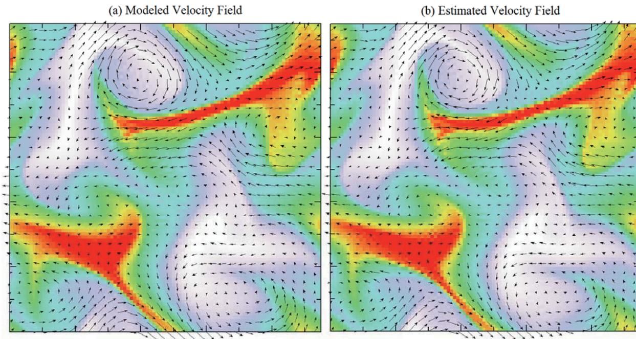
Figure 2. Velocity fields: (a) and (b) Average of the actual vector fields generated by the model at time  $t_1 = 18$  hr and  $t_2 = 20$  hr. (b) Estimated vector fields obtained by the new nonlinear inverse model from an image sequence between  $t_1$  and  $t_2$ .
