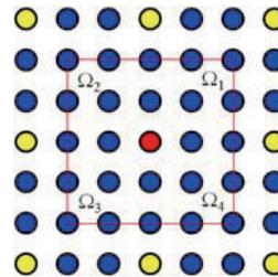
Figure 1. Bilinear square pixel sub-arrays ( $n_x = 3$  and  $n_y = 3$ ) with 9 node points in which yellow ( $p, q$ ) and red ( $k, l$ ) node pixels are unknown velocities that are mapped onto an image scene.
