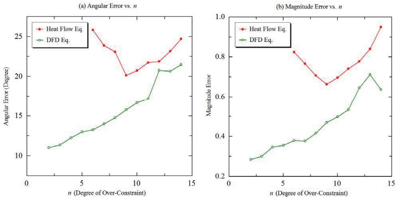
Figure 3. Plots of error measurement generated by the linear and nonlinear inverse models with numerical model data at time  $t_1 = 18$  hr and  $t_2 = 20$  hr: (a) Mean values of angular error defined by the equation (11) vs.  $n$  (a degree of over-constraint), and (b) mean values of magnitude error defined by the equation (12) vs.  $n$ .
