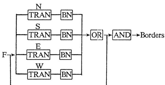
Fig. 3 Block Diagram for Border Following
