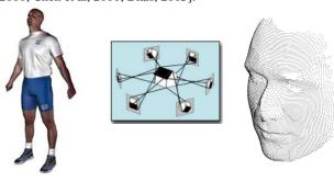
Figure 1: 3D model of human produced with a Cyberware Body Scanner [11] (left). A bundle adjustment solution for multi-image photogrammetric reconstruction (center; Source: Photomodeler [31]). A point cloud generated with a matching algorithm on 5 images (right) [D'Apuzzo, 2002].
