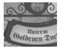
Figure 8: Same as Fig. 7, but with a digital camera using a Dalsa CCD chip with 6 Mega-pixels. On the object, each pixel represents the same 7mm as in Figure 7.
