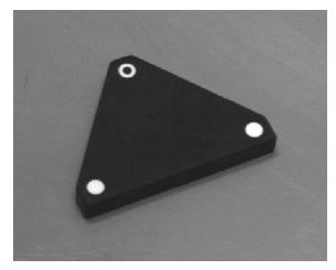
Figure 3. Calibration tool.
