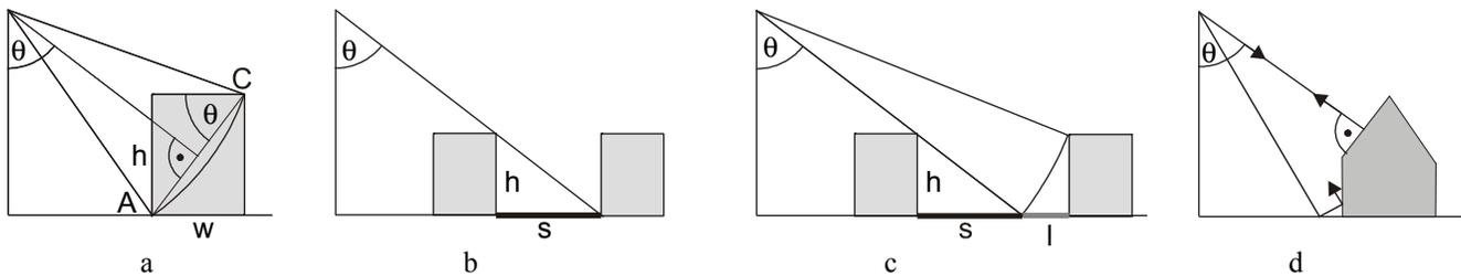
Fig. 7. Geometric constraints for the acquisition of SAR images from buildings.
