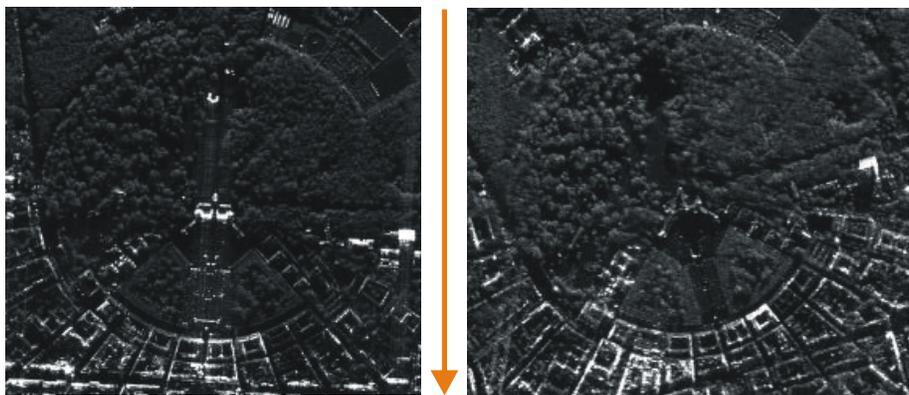
Fig. 8. Two SAR images taken from different flight paths. The arrow shows the range direction. The set of buildings (segment of the circle) which shows strong reflections differs in both images.
