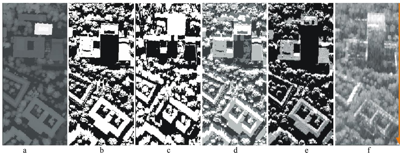
Fig. 9. a) Laser elevation data, b) shadow simulation, c) layover simulation, d) SAR phenomena image with shadow and layover, e) Simulation of SAR image, f) SAR image
