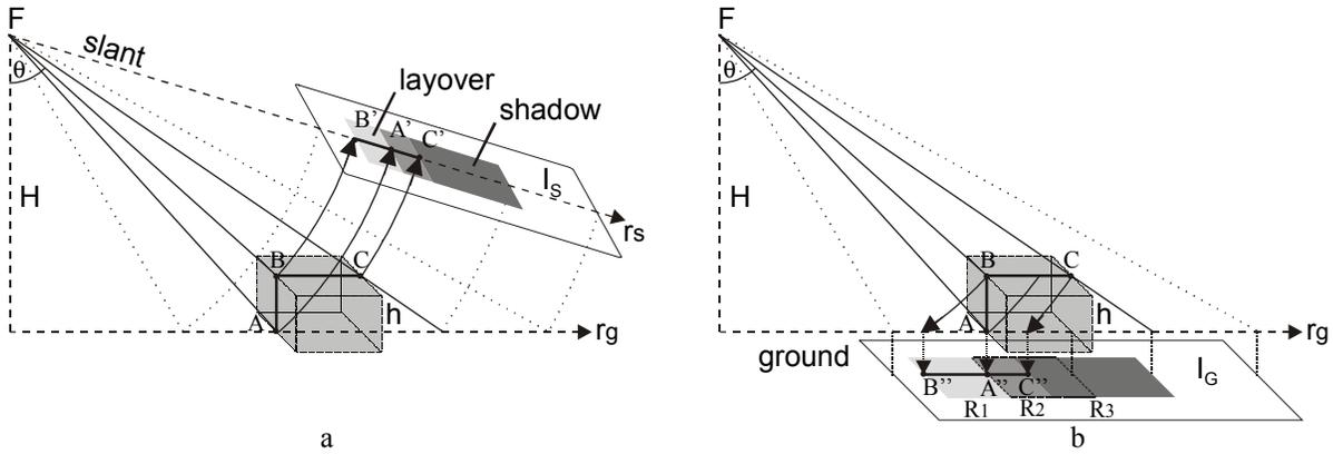
Fig. 4. Projection of a building into a) slant image ( $I_S$ ) and b) ground image ( $I_G$ ).
