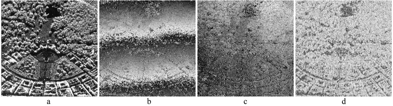
Fig. 3. Slant image (test area Karlsruhe). a) intensity, b) phase difference, c) elevation, d) coherence,
