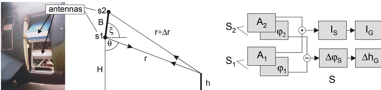
Fig. 2. SAR system AER II, geometry of across-track interferometry, and signal processing.
