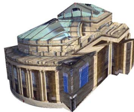
Figure 8. Building model automatically textured without occlusion culling.
