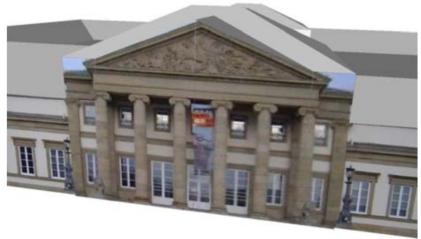
Figure 5. The 3D building model with the extracted textures placed on the façade polygons.
