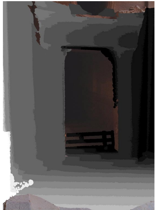
Figure 7. The distance image of the left door projected on the corresponding image.
