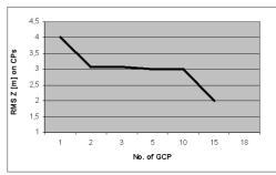
Figure 5. Altitude accuracy (on control points) for generation of DSM depending on a number of GCP in environment Photomod
