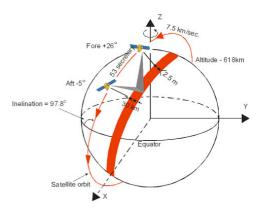
Figure 7. Elements of the orbit of system Cartosat-1.
