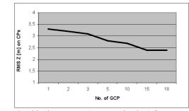
Figure 3. Altitude accuracy (on control points) for generation of DSM depending on a number of GCP in environment PCI Geomatica
