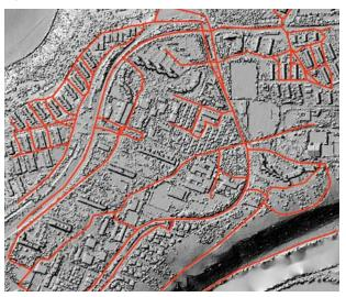
**Figure 11.** The extracted road network overlaid on the laser point cloud (red-road centerlines, background- shaded relief of the laser point cloud).
