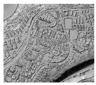
Figure 8. Shaded relief of the laser point cloud.
