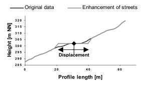
Figure 6. Cross-section of the original DTM with and without the enhanced street.
