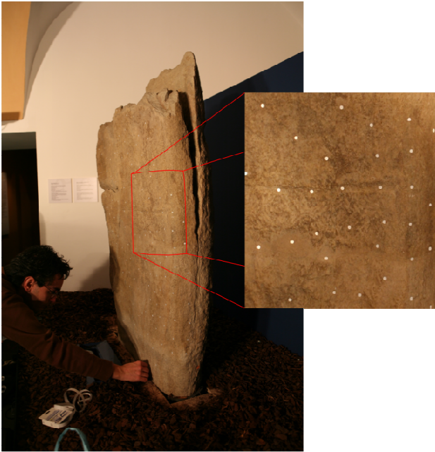
Figure 5. Placing the reflective targets on the object
