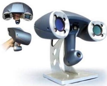
Figure 3. Handyscan 3D: the acquisition unit (980 g, 160 x 260 x 210 mm, ISO accuracy: 20 \mu m + 0.2L/1000)
