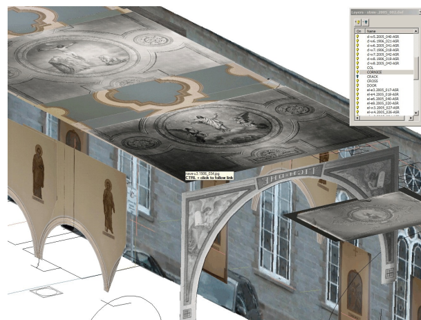
A part of the finished 2½D photomosaic as a DWF showing Layer control and a Hyperlink to the source image.
