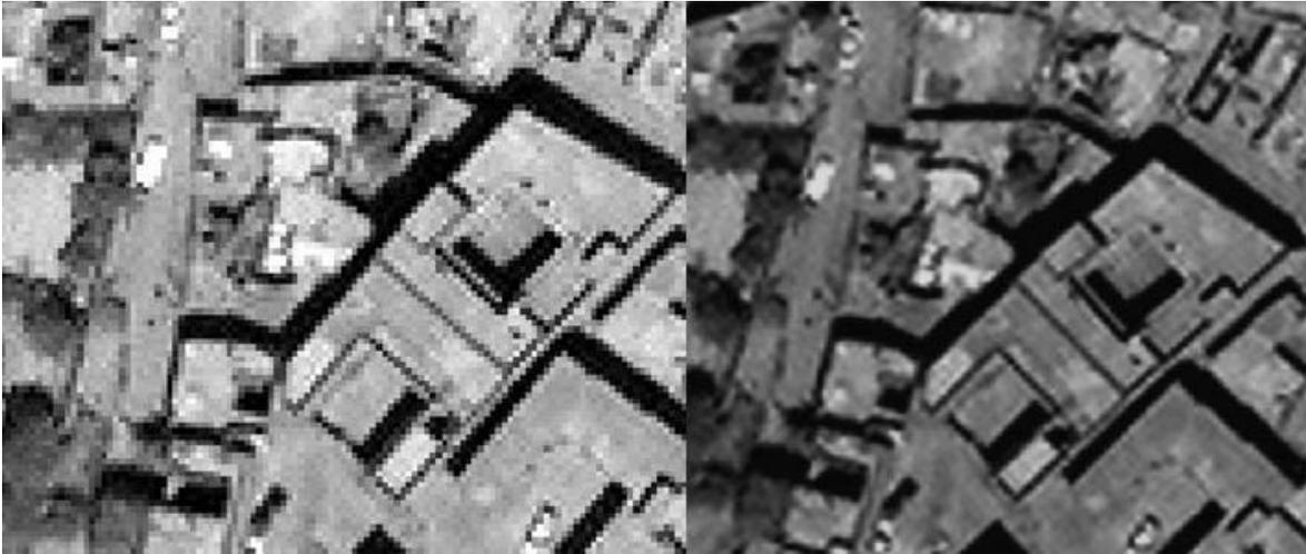
Figure 9. Image enhancement (left: original satellite image, right: filtered image)
