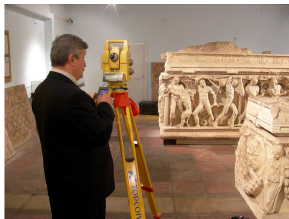
Figure.2 Total Station and measurement of sarcophagus
