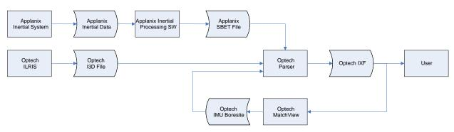
The resulting Optech IXF file contains a fully geo-referenced point cloud data set in WGS84 coordinates.
