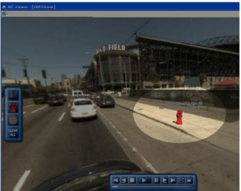
Figure 6: An augmented immersive image. The fire plug is a virtual geo-referenced object inserted into the scene.
