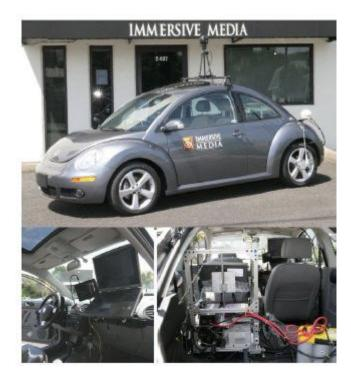
Figure 5: Telemmersion® data collection vehicle with Applanix POS/LV 200 navigation system
