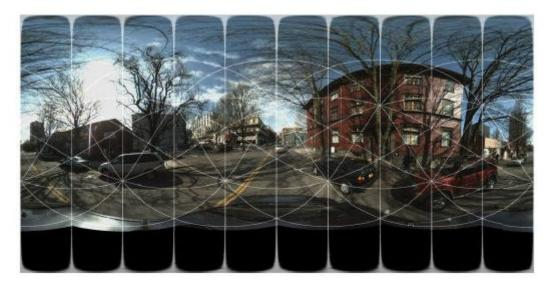
Figure 2: Stitched panoramic image with lines connecting sensor focal points superimposed.
