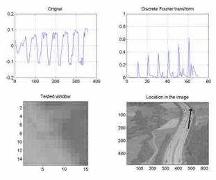
Figure 4. Example for an interest location of the T-class: For each radius the lowest frequency dominates (180° structure). For the larger radii this gets stronger
