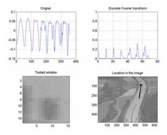
Figure 5. Example for an interest location of the vehicle cue class: Spot structure leads to reduction of features for larger radii, for the very large radii disturbance from surrounding occurs
