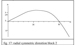
The systematic image errors of block 1 and block 2 are similar. This is guaranteeing that the influence of the control points is negligible for this. If the camera geometry is stable, the systematic image errors determined in one block could be used as a camera calibration. By this reason in a second step, the image coordinates of block 2 have been corrected by the systematic image errors of block 1
