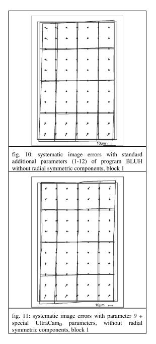
The block adjustment has been handled in tangential coordinate system to avoid problems with the earth curvature. In addition the image coordinates are improved by standard refraction correction. Nevertheless the radial symmetric component is dominating the systematic image errors. The influence without the radial symmetric component is shown in figure 10.
