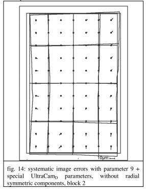
The second block shows the same trend of the systematic image errors like the first block. Of course the values are not identical because of the influence of random errors.
