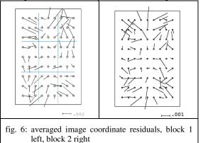
Both blocks show the same tendency of systematic image errors based on block adjustment without GPSvalues of the projection centres and without selfcalibration by additional parameters.
