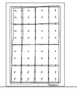
fig. 12: systematic image errors with standard BLUH parameters + special UltraCam<sub>D</sub> parameters, without radial symmetric components, block 1
