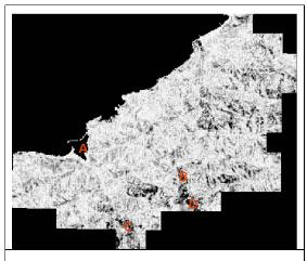
Fig. 1: grey value coded height differences SRTM Xband height model against reference DEM white = 0.0m, black  $\geq$  30.0m or no data
