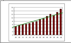
Fig. 2: root mean square height differences SRTM X-band DSM against reference DEM for open areas as function of terrain inclination
