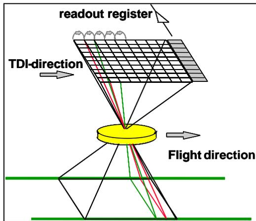
Figure 2. digital forward motion compensation
