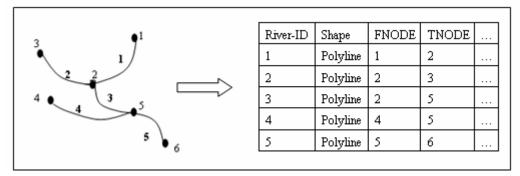
Figure 5. The attribute table constructed by calculating topology structure
