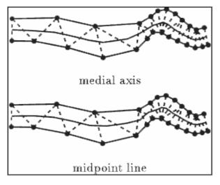
Figure2. The medial axis and the midpoint line approximation.
