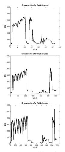
Figure 8 - Radiometric response of the panchromatic channel from three images from the same object area and different GSD
