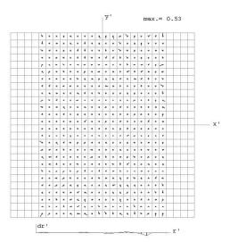
Figure 9 - Remaining image residuals less than 0.53  $\mu$ m after the least squares adjustment including additional self calibration parameters
