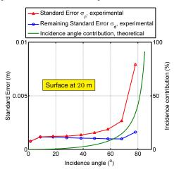
Figure 4: Measurement precision with respect to the incidence angle of the surface, given a fixed scanner position. The standard total error  $\sigma_{\rho}$  is plotted in blue. In green is plotted the theoretical noise induced by the incidence angle. The remaining standard error  $\sigma_d$ , after removal of the incidence angle effect following Eq.10, is plotted in red.
