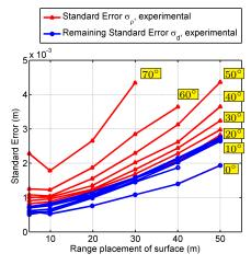
Figure 6: Measurement precision with respect to the range placement of the surface. The standard total error  $\sigma_{\rho}$ , *i.e.* the RMSE of the residual to a plane fitting, is plotted in blue for each incidence angle experiment at each range placement. Each rotation experiment is labeled with the incidence angle. The remaining noise, after removal of the incidence angle effect per point, is plotted in red for each incidence angle experiment at each range placement.
