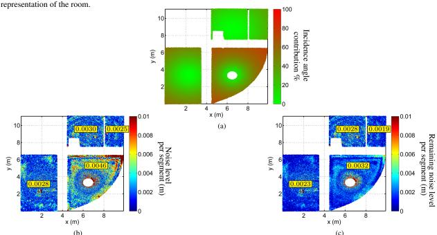
Figure 8: Net view of the point cloud of the room: (a) Incidence angle contribution, (b) Noise level  $\hat{\mathbf{e}}_{\rho}$ , *i.e.* the residual to a plane fitting. Standard error value of the four main segments is plotted, (c) Remaining noise level  $\hat{\mathbf{e}}_{\mathbf{d}}$ , *i.e.* the residual to a plane fitting after removal of the incidence angle effect. Standard error value of the four main segments is plotted.
