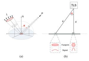
Figure 1: Schematic illustration of the reflection geometry. (a) Incidence angle of the transmitted laser beam with respect to a surface. (b) Perpendicular and incident laser beams with respect to a planar surface. The footprint shape and the reflected signal are plotted for the perpendicular and one slanted situation.
