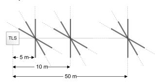
Figure 5: Top view of the measurement setup 2, with schematic depiction of distance placement of the plate with respect to the TLS.
