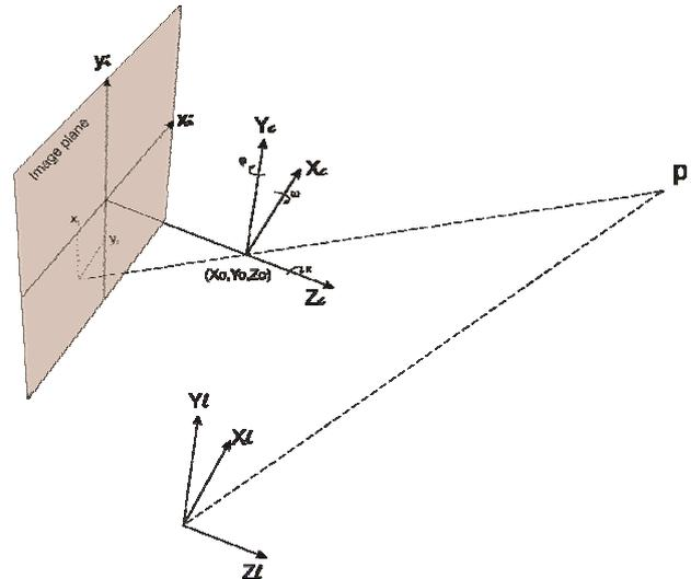
Figure 1: Laser scanner – image coordinate systems
