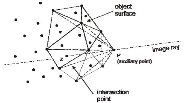
Figure 3: Ray intersection directly to the point cloud
