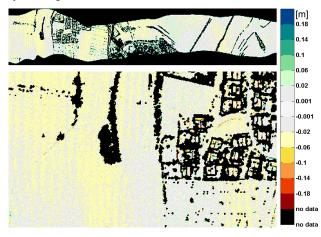
Figure 7: Strip differences for the improved georeferencing after the strip adjustment; cf. fig. 6. Note that the systematic patterns of the height differences, which are visible in fig. 6 (especially at the roofs), have now disappeared to a very high degree.
