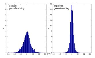
Figure 5: Histogram of the strip differences  $dZ_{pair}$  (considering the roughness mask) based on all overlapping strips (ca. 118 million values). Left: original georeferencing ( $\sigma_{MAD}$ =6.2cm). Right: improved georeferencing after strip adjustment ( $\sigma_{MAD}$ =2.9cm).  $\sigma_{MAD}$  is the standard deviation derived from the median of absolute differences (the so-called *MAD*) as  $\sigma_{MAD} = 1.4826 \cdot MAD$ .
