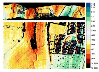
Figure 6: Strip differences for the original georeferencing. Top: Overview of a color coded difference of two overlapping strips. Bottom: Enlarged detail; observe especially the striking red and blue patterns at the roofs (with height differences beyond  $\pm 18$ cm). These are caused by horizontal errors between the two strips. Right: Legend of color coding. Black is used for the area outside the overlap of both strips, but also for the parts covered by the roughness mask.
