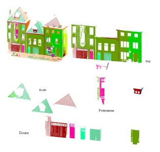
Figure 1. Semantic feature extraction from terrestrial laser scan
