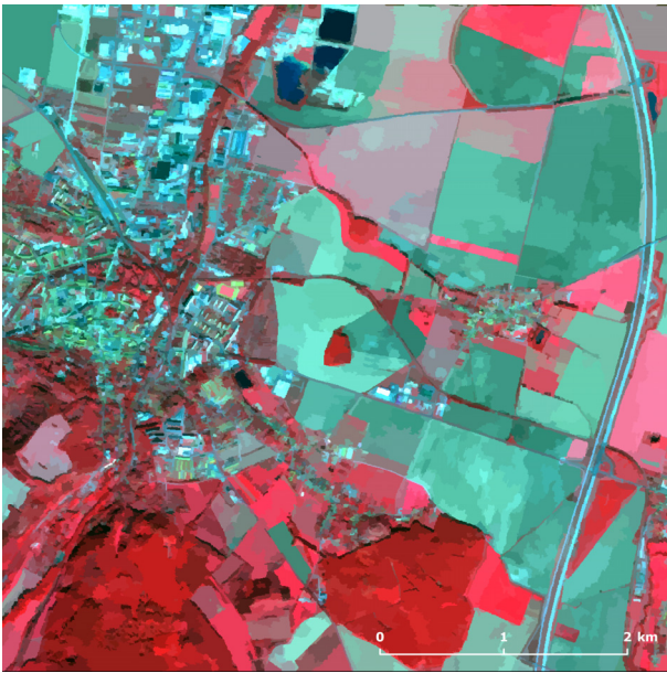
Figure 2. Sample result for the image segmentation combining region growing and watershed transformation approaches. Image segments are coloured using the average values in the near-infrared, red and green bands, respectively.
