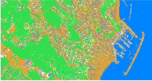
Figure 2. Portion of classification results for test L0-D1-A near a small harbour: V=green, A=orange, W=blue and B=grey, NC=white.
