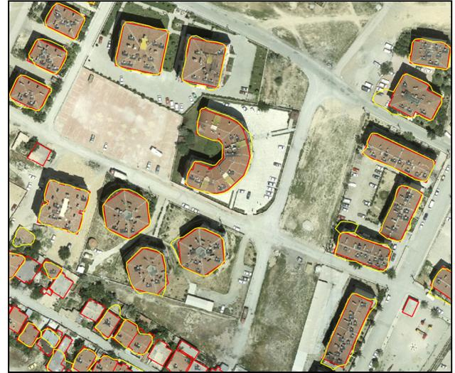
Figure 2. A small part of the ortho-image. The red polygons show the available reference data, the yellow polygons shows the results of the proposed methodology.
