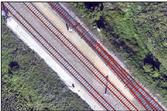
Figure 3. Rail track extraction result using Feature Analyst
