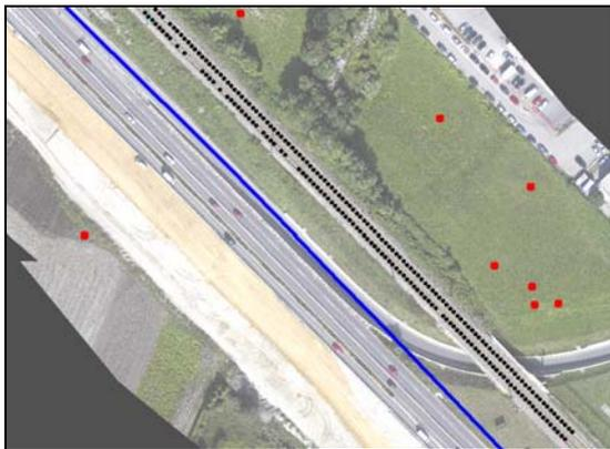
Figure 10. Resulting track axis points (black) along the trajectory (blue), outliers are coded in red
