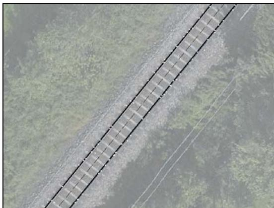
Figure 6. Ortho-image overlaid with the extracted rail tracks: rail (solid), rail centre line (dashed) and filtered rail points (white) (right)
