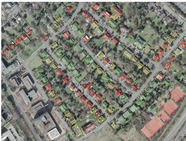
Figure 10: Reconstruction results on the "Gronau" data set. Buildings fully automated reconstructed are depicted in green. Reconstructions obtained by the semi-automated approach (cf. text) are depicted in yellow. Reconstructions obtained by interactive indexing (cf. text) are depicted in red.
