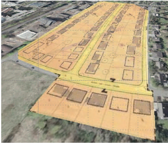
Figure 7: Perspective on our benchmark data set showing DSM layer textured with the aerial imagery layer data and overlaid with a development plan.
