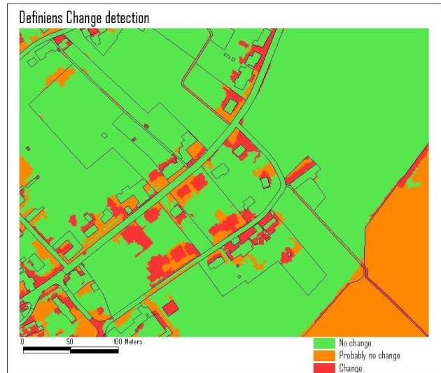
(b) Definiens change detection: comparison DB0 and Definiens classification (change=red; probably no change=orange; no change=green)
