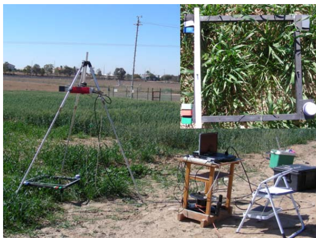
Figure 1. Spectral Camera HS in a wheat field, focusing on the sensor point of view - the frame including wheat and GW as well as BLW.
