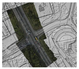
Figure 4. Vector data and ortho photo on the top of the elevation model. All data sets were transformed in the same coordinate system.
