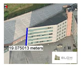
Figure 8. Obtaining height values from Pictometry application.
