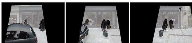
Figure 3. Example of laser-based occlusion layers superimposed with the corresponding rectified images.
