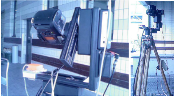
Figure 1: The panoramic images acquisition system. It can support any kind of camera.
