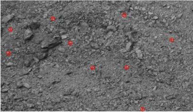
Figure 2. Control points spread around rock glacier.
