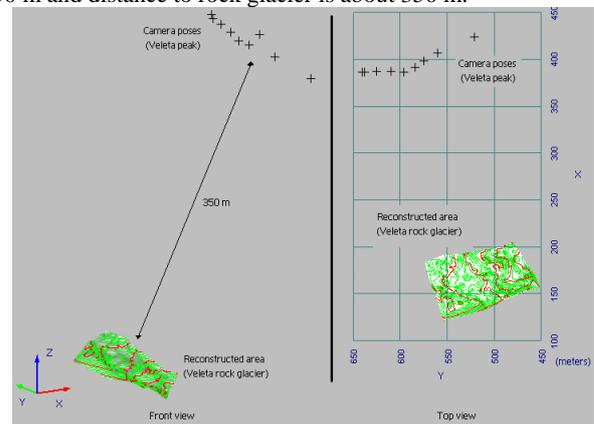
Figure 1. Camera situation respect the reconstructed area
