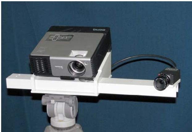
Figure 1. The projector-camera photogrammetric system
