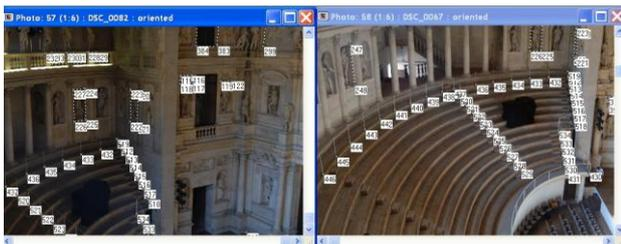
Figure 4. Example of matching point extraction.
