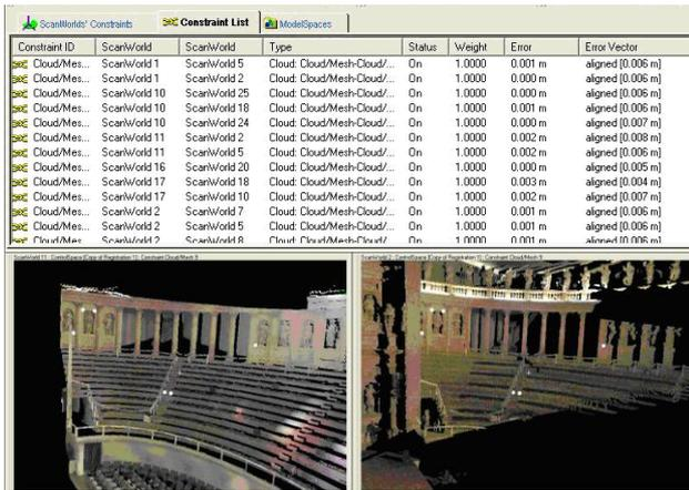
Figure 7. Pairwise scan alignment.
