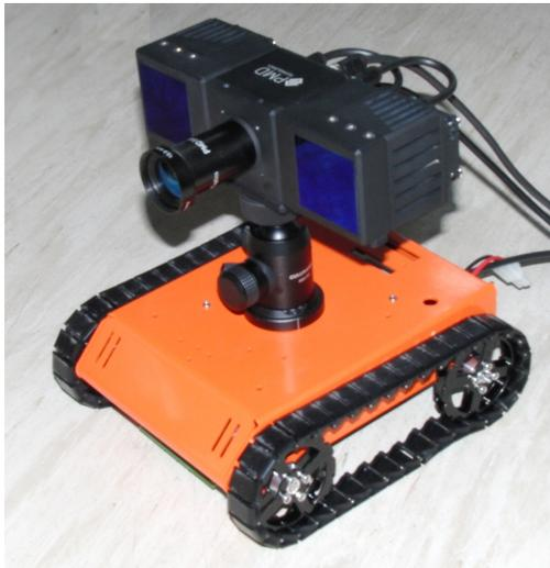
Figure 1: Used mobile robot with PMD CamCube 2.0
