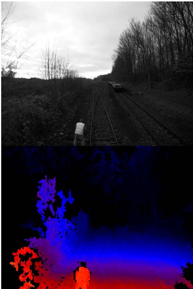
Figure 4. E3D experiment on a railroad engine, one image of the stereo camera system (top), disparity image (bottom)
