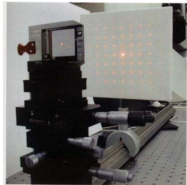
Figure 2. Projection of patterns generated by a diffractive optical element to a screen
