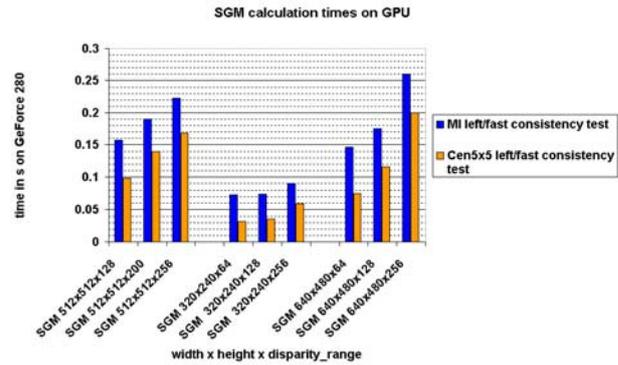
Figure 5. Computing times for different GPU's, image sizes and cost functions
