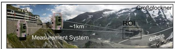
Figure 4: Panorama of measurement site at the Pasterze glacier, including scanning position (left) and region of interest (ROI) on the object (area covers about 370m x 120m)
