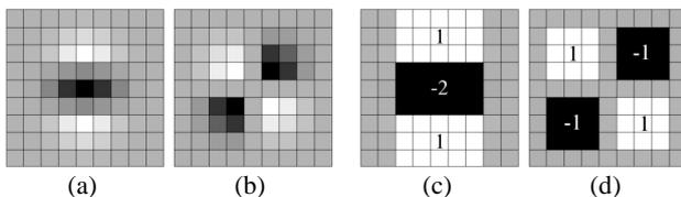
Figure 2: Filter kernel for the second derivation of the Gaussian (a and b) and crude approximation through box-filters (c and d) (Bay et al. 2006).
