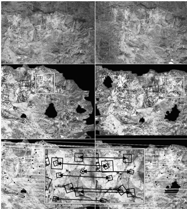
Figure 3: Operator Test, *top*: original 12MP stereo images, *middle*: interest points in masked area including descriptor size and orientation of matches (framed sample sub-region), *bottom*: zoomed out sub-region showing homologue points (including descriptor window) connected by arrows (background displays all other matches)
