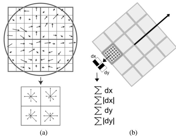
Figure 1: (a) SIFT: aggregation of histograms of oriented gradients (LOWE 2004); (b) SURF: 4 descriptor vector values gained from each of the 5x5 wavelet responses (EVANS 2009).
