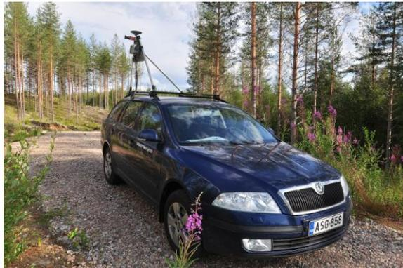
Figure 4: The MMS system mounted on car
