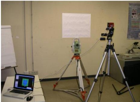
Figure 1. System adopted to study the influence of “scattering” on the camera distance measurements.
