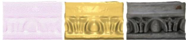
Figure 13. ToF Point cloud (left), mesh (centre), textured final model (right).
