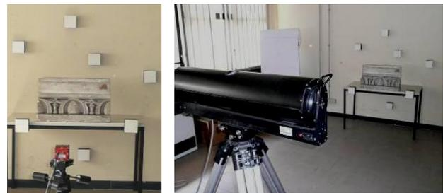
Figure 11. Data acquisition of a frieze with the SR-4000 camera and the Riegl Mensi S10 laser scanner.
