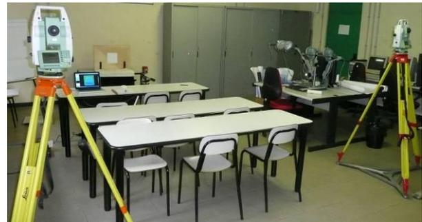
Figure 9. Topographic measurements for the estimation of camera and tested object positions.
