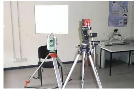
Figure 5. System used to evaluate the influence of the alpha angle on camera distance measurements.
