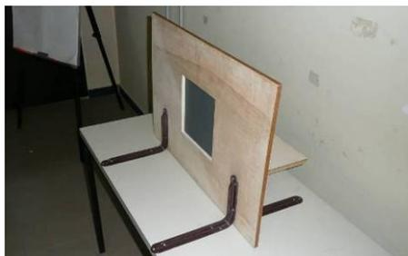
Figure 8. Purpose-built system for positioning planar objects of different dimensions.
