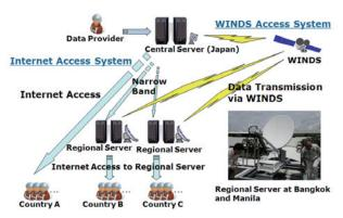
Figure 6. Sentinel Asia Step 2 system using WINDS
