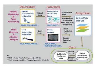
Figure 4. Concept of Sentinel Asia flood monitoring. SA provides accumulated precipitation data and inundated area information observed by satellite on the Web-GIS. This figure is provided courtesy of K. Fukami of ICHARM.
