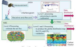
Fig. 6 Data Processing Flow
