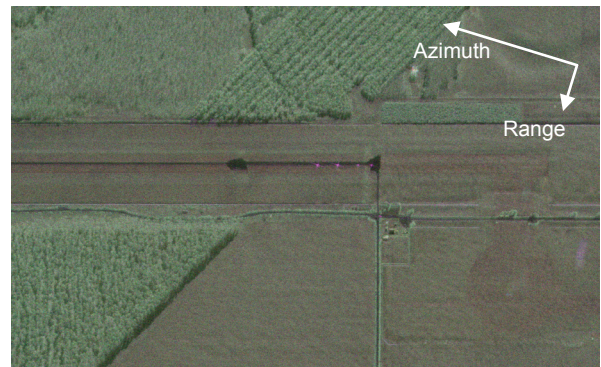
Figure 10. Pi-SAR2 model RGB power composite image (R:HH, G:HV, B:VV)( \times 10/2/2 ). Incidence angle is about 42deg. The runway and surrounding area were covered with 50 cm-depth dense snow.
